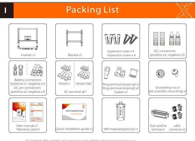
AC terminal x8 \*: 4 6AWG AC terminals and 4 10AWG AC terminals for Version I 4 10AWG AC terminals and 4 8AWG AC terminals for Version E and Version C
