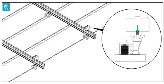
> Attach the end-clamps to the edge of the module field on the mounting rails.
