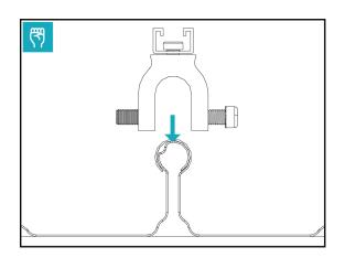
Attach the round seam standing seam clamp to the roof seam.
