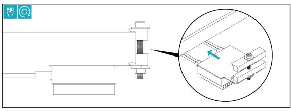
[>] Install the microinverter onto the module according to the module manufacturer's instructions.
