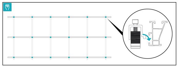
Attach a cross connector to the upper rail for each cross connection.
