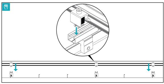
> Attach the cross connector to the short rail in each case.
