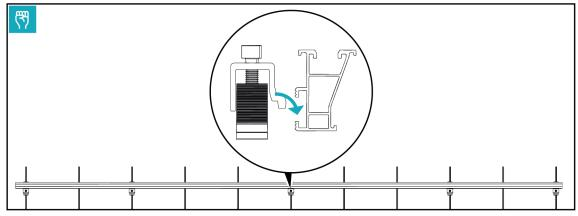
> Attach a cross connector to the mounting rail for each short rail in a row.
