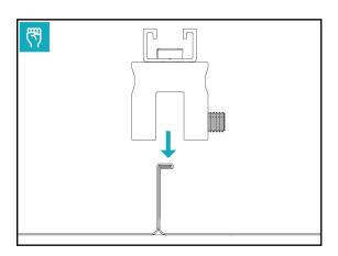
Attach the single-folded standing seam clamp to the roof seam.
