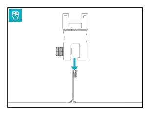
Attach the double-folded standing seam clamp to the roof seam.
